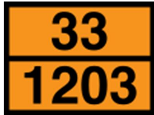
Figure 2 - Orange plates used in ADR transport for single material, in these case - petrol
